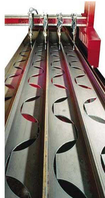
Figure 8: Cutting of a Cellular Beam
